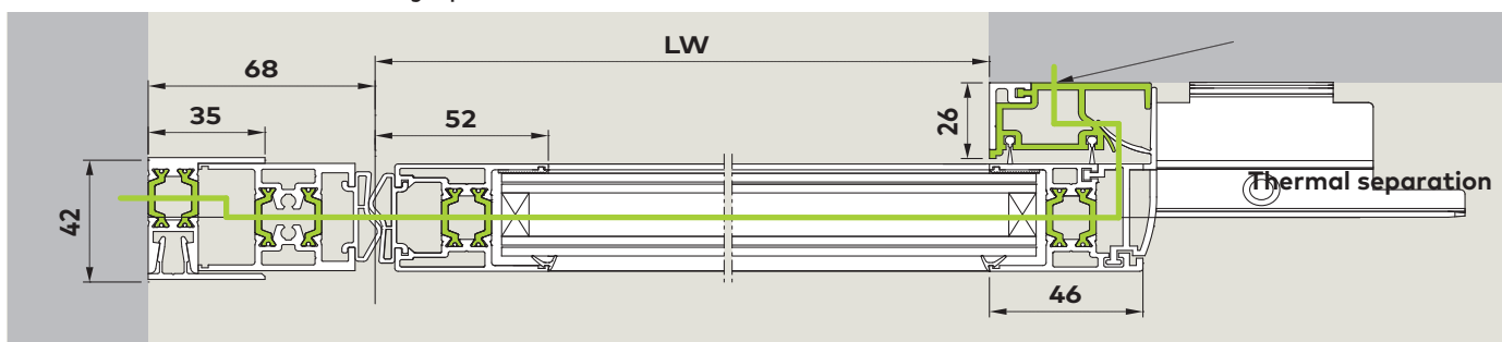
Horizontal section of lintel-mounted single-panel version
