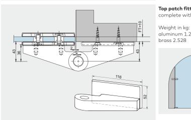
Top patch fitting complete with pivot for sidelight
