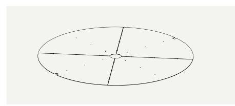
Stainless steel plate for floor element – perforated (for drainage)
