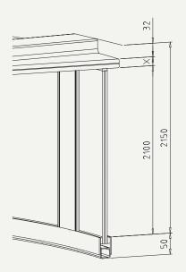
If the RDR-S01 is installed in the facade axis, we recommend providing additional weather protection using a roof with an appropriate downward slope
