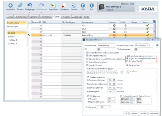
The powerful software allows the complete Paxos® advance IP system to be configured. Additionally, the software contains an online monitor as well as an area for reading out the audit trail.
